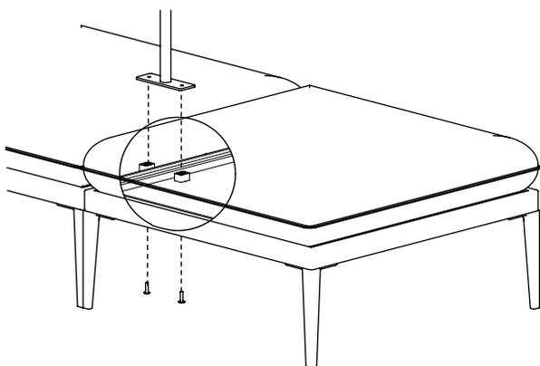
Place 2 x 3/4" blocks between the seat board and the shelf so that everything is level. Insert 2 1/4-20 x 1.75" round head screws under the seat board, through the blocks to secure the shelf between the seats.
