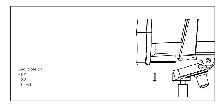
**IMPORTANT:** Note that the screws are already inserted in their proper holes. (Unscrew them and rescrew in position with a hammer drill)
