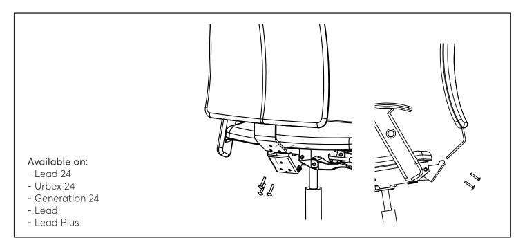
**IMPORTANT:** Note that the screws are already inserted in their proper holes. (Unscrew them and rescrew in position with a hammer drill)
